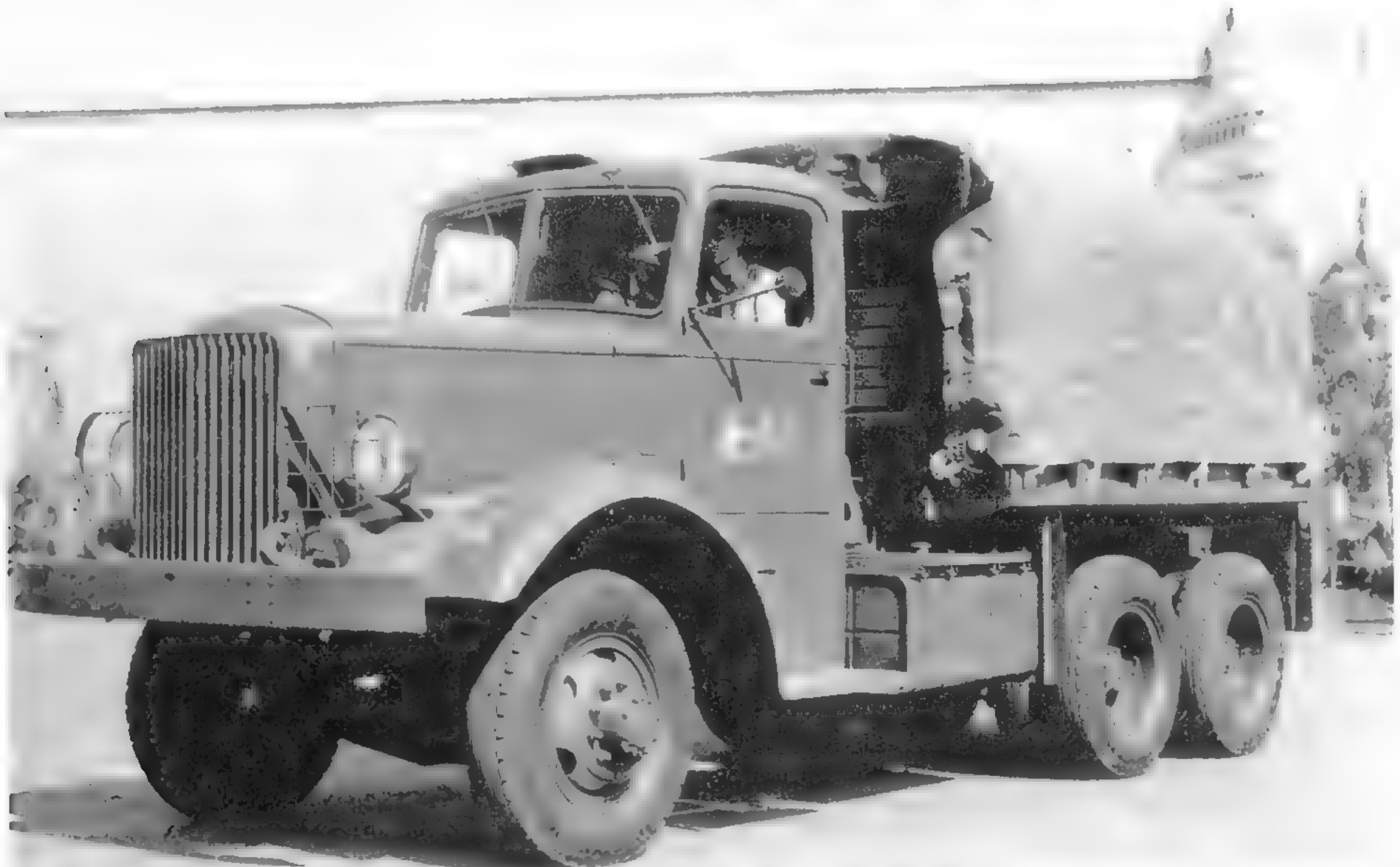
The Mack NM-1 (shown here), NM-2, and NM-3 trucks were supplied with Lee tires with highway tread. Initially, the size was 9.75 x 22 in., but soon that was increased to 10-22. The NM-1 and -2 had a flat bumper with tow hooks mounted on the top. (Photo courtesy of the Mack Trucks Historical Museum)
